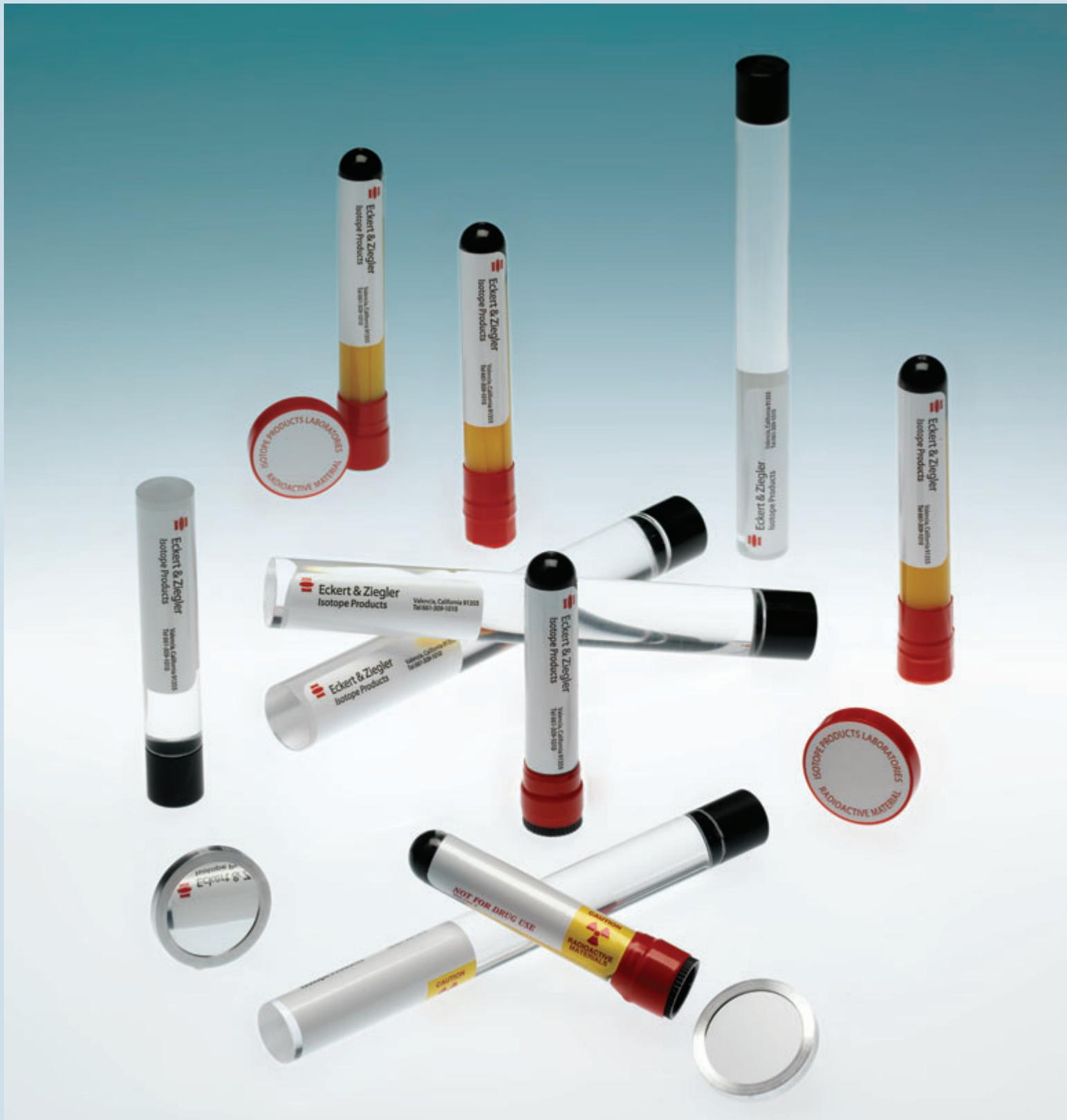
A wide range of gamma and x-ray standards for research and educational use are available in the energy range of 5.9 to 2614 keV. Many nuclides are available up to 100  $\mu\text{Ci}$  (3.7 MBq) to allow for the lower efficiencies of detection inherent in many instruments. Available activity ranges are listed for each nuclide in the tables on pages 46 to 53. Please contact customer service for other activity requirements.
