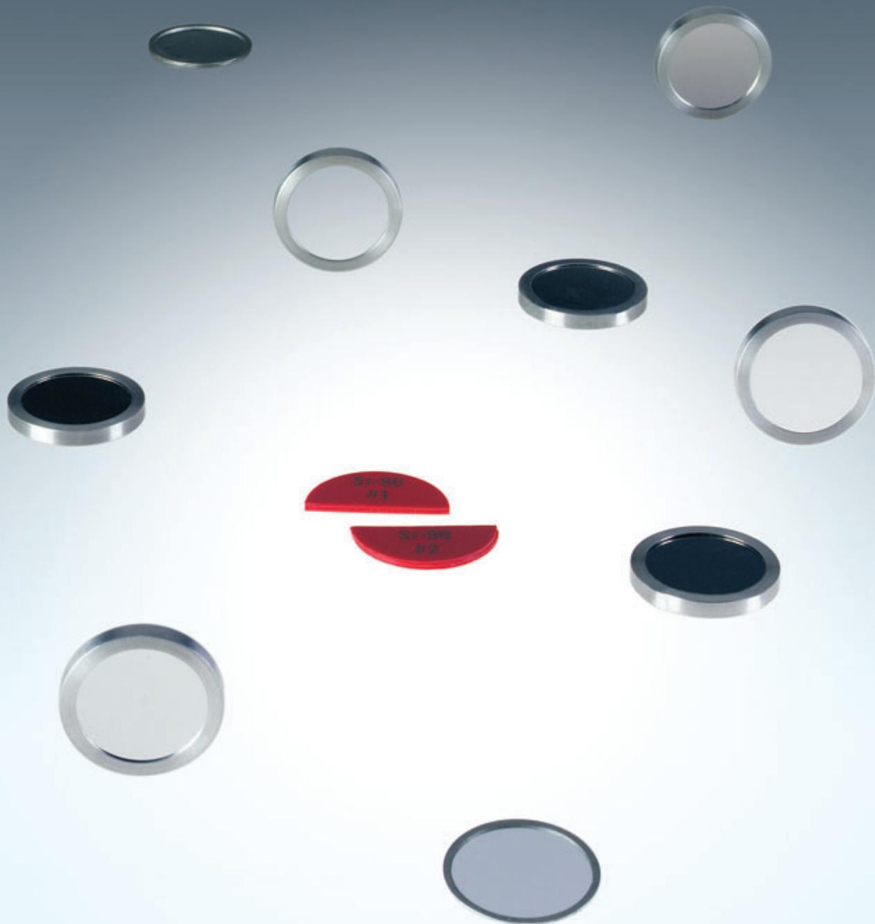
A wide range of beta emitting nuclides are offered for counting and educational uses. Certification of all BF Series sources includes both contained activity and 2π emission rate. Sources are traceable to NIST with ±2% to ±5% accuracy at the 99% confidence level. Source configurations are surface conductive on all surfaces to enable their use in windowless proportional counters.
