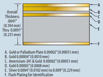
**Figure 67-B : Po-210 Rolled Foil Cross-Section**
